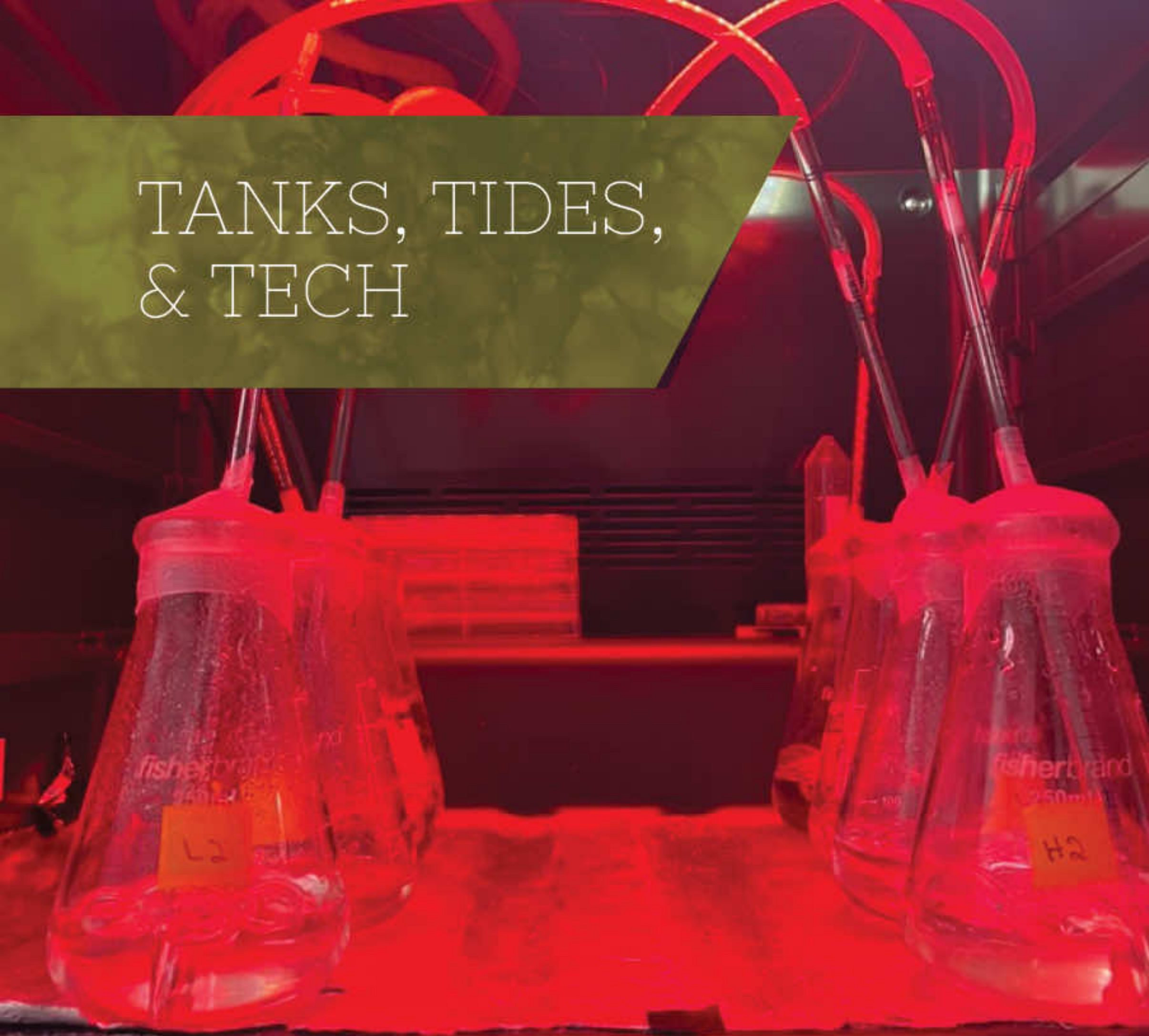
▲ Spore germination experiment based on starting density of cultures
